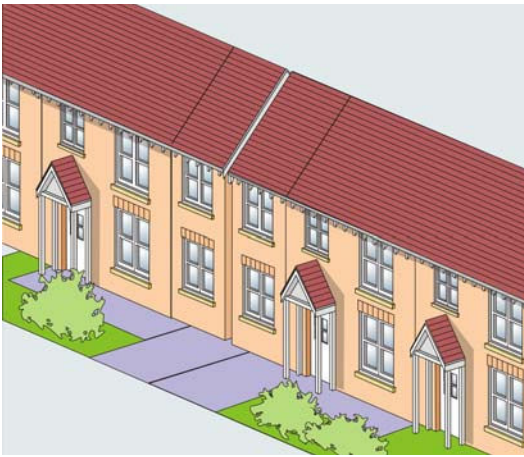
Diagram 11: Inappropriate side extensions which have led to a 'terracing effect'
