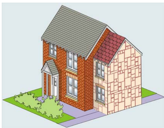
Diagram 1: Poor choice of external materials for the extension
